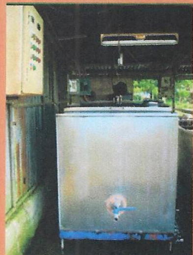
COOLING TANK Capacity : 1,000 Liters Storage : Up to 3 days
